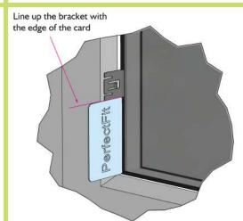
To ensure all the brackets are in the correct position for fitting (85mm from beading) use a credit card in the corner of the window to locate the bracket position.
