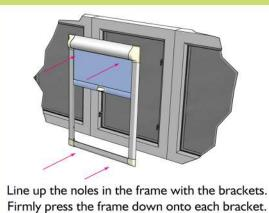
Fit one side at a time for easier installation.
